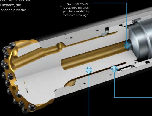
ALL AIR FLUSH THROUGH THE SPLINES Maximized cooling and lubrication of the splines eliminate the risk for bit shanking, resulting in higher productivity through increased reliability.
